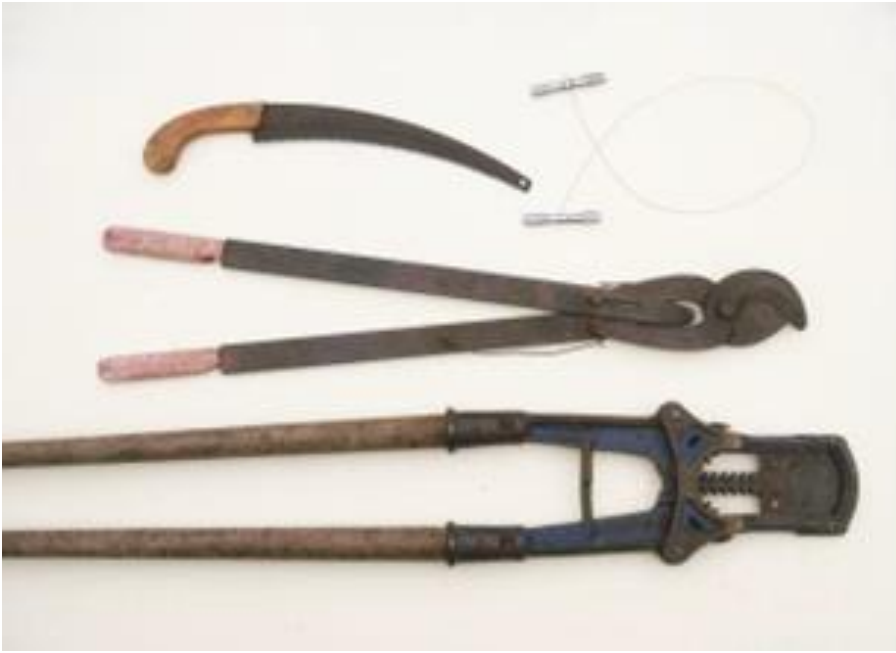
Image 5 – Instruments for horn tipping. Horn saw (top left), embryotomy wire (top right), parrot nose horn tippers (middle), guillotine dehorner (bottom). Guillotine dehorner will not fit over an ingrown horn therefore unsuitable. Source: Meat and Livestock Australia.
