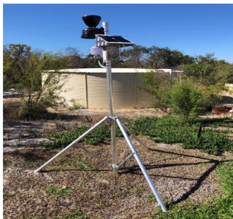
Figure 5: Tripod with electronics box, sensors and solar panel
